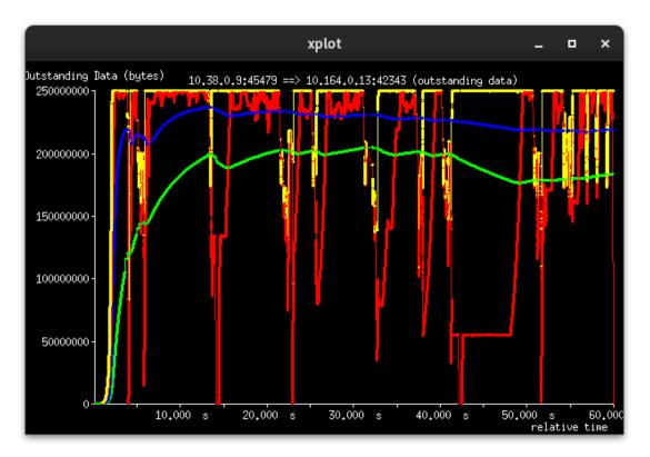
This is a much busier chart. BBR does not react to packet losses in the same way Cubic does. It is going to look at the changes in round-trip-time and achieved throughput when deciding on a congestion window. You can see that for this run, by and large the Red line remained above 50,000,000 bytes where Cubic never got that high. There were also times when it had indeed filled the receive window of 256 MiB.
